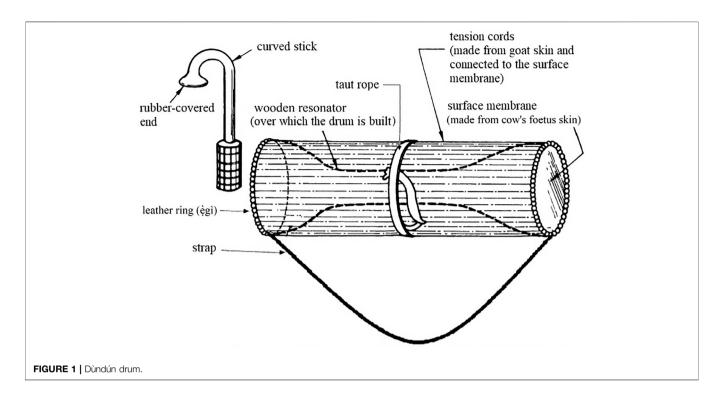
The drum is played with a curved stick. To avoid puncturing the drum, the head of the stick is covered with a flat rubber or leather material. To carry the drum, a strap is made from leather and padded cloth. Depending of the handedness of the drummer, the drum is suspended over the left or right shoulder with the strap and hangs under the opposite armpit.
