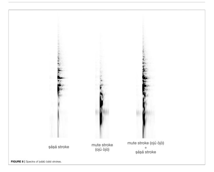
drumheads to merge. This is noticeable on the spectrogram images of the different  $iy\dot{a}\dot{a}l\dot{u}$  bàtá stroke combinations, showing that the frequency spectra of the sásá and the  $oj\dot{u}$   $\dot{o}j\dot{o}$  membrane do overlap each other partially on the mid region. Thus, more than simply combined, the two independent membrane sounds can be said to be acoustically intertwined.
